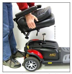
Figure 14. Removing the Seat
