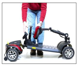
Figure 20. Connecting Frame and Drivetrain
