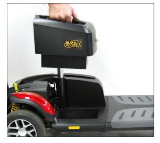
Figure 21. Battery Pack Installation
