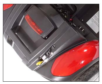
Figure 11: Freewheel Lever (Drive Position)
