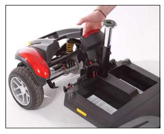
Figure 17. Separating the Drivetrain and Frame
