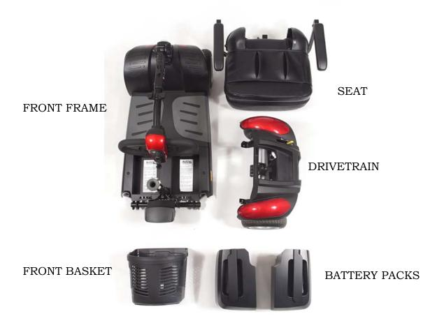
Figure 18. Buzzaround Extreme<sup>TM</sup> Components (Model GB148EX)
