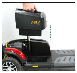
Figure 15. Removing the Battery Pack
