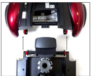
Figure 19. Drivetrain Alignment
